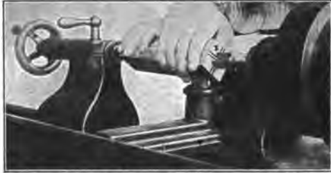
Fig. 5. Placing a Piece Between the Lathe Centers.
